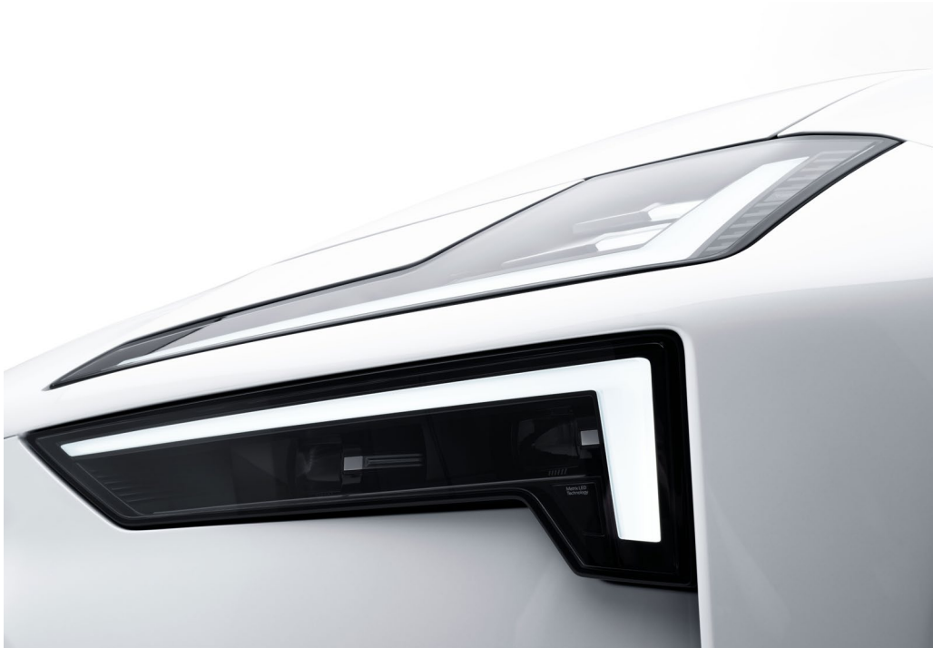
Pixel LED headlights Individually controlled Pixel LEDs that automatically adapt to the surroundings. Available as an option.
