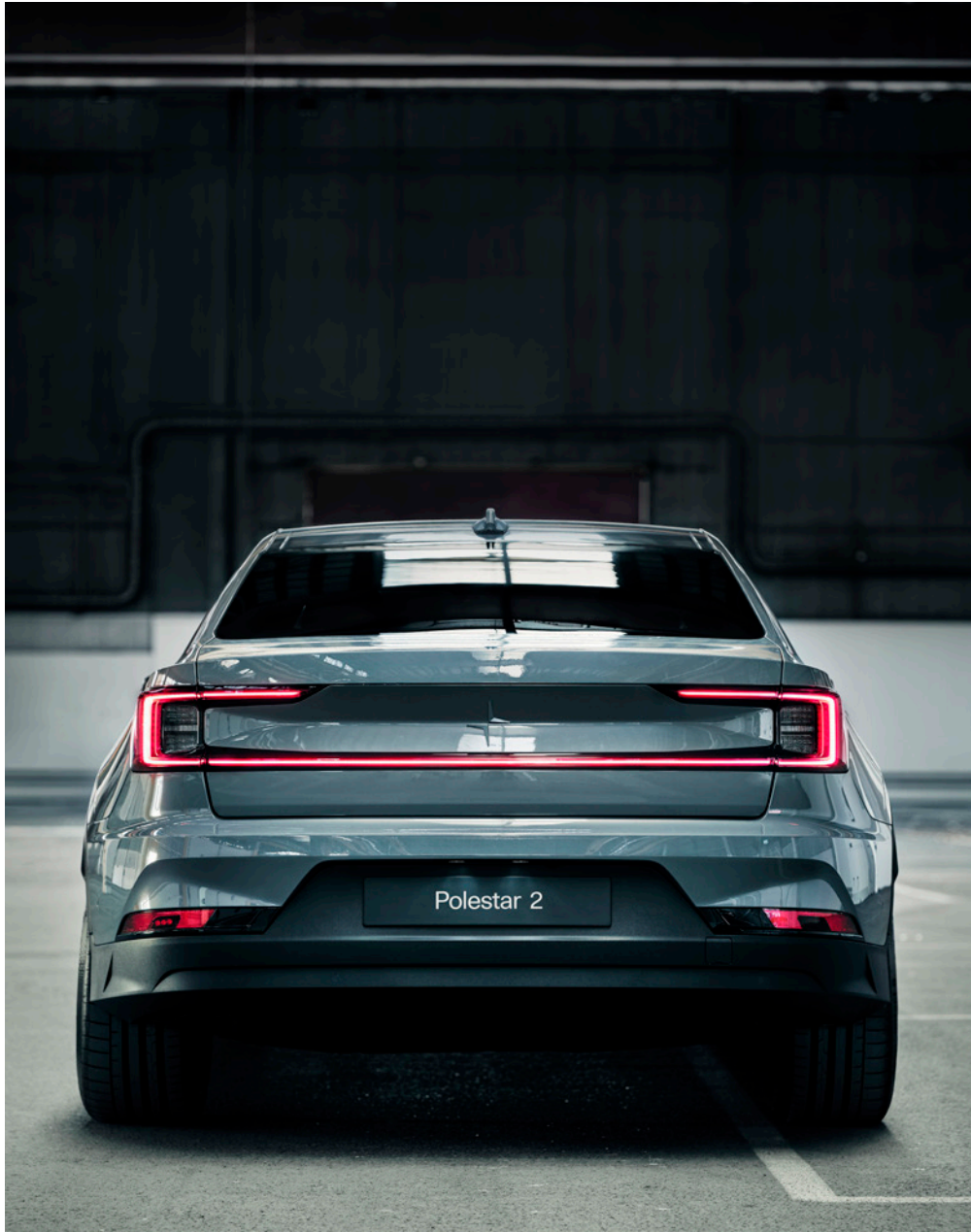
The rear crystal light blade uses 288 power LEDs to give the rear of the Polestar 2 a unique fullwidth light signature.
